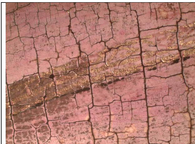
Image 4: During Treatment stereomicroscope image of Saint Catherine showing removal of the patches of dark coating.
